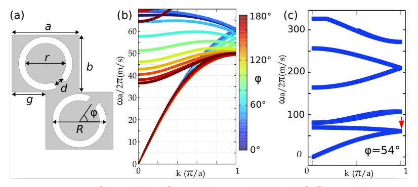
b = 0.85a, d = 0.15a, r = 0.3a, and R = 0.4aHard-wall boundary conditions to define a waveguide
