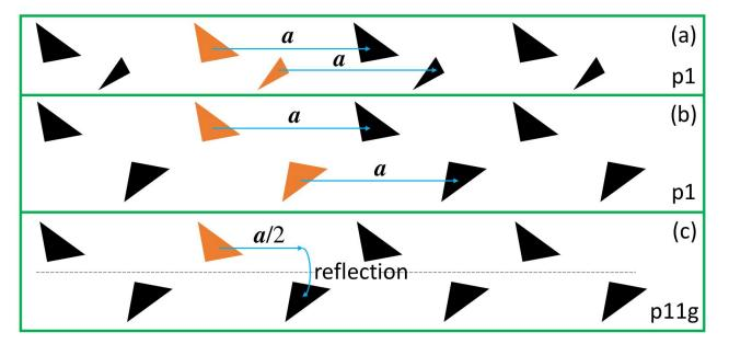
Glide-reflection symmetry reduces the lattice constant by a factor 2 (band folding), resulting in a gap closing
